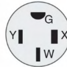
50-A, 125/250-V, 3-POLE, 4-WIRE, GROUNDING TYPE
