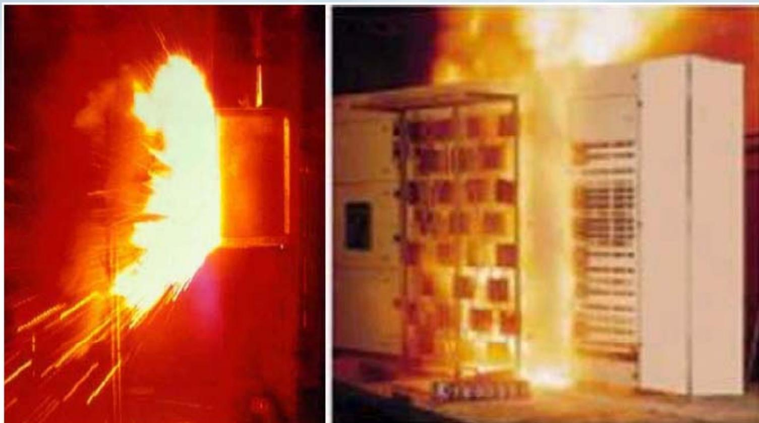
Figure 1.1: (a) Arc blast in box<sup>2</sup> ; (b) Arcing fault in electrical panel board
