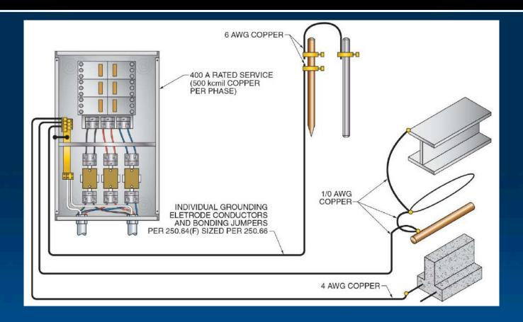
New text was added to 250.66(A), (B), and (C) to clarify that if the grounding electrode conductor or bonding jumper connected to a specific electrode does not extend on to other types of electrodes that require a larger size conductor, the grounding electrode conductor(s) shall not be required to be larger than the sizes specified at 250.66(A), (B), and (C)
