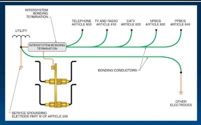
**250.94(A)** The Intersystem Bonding Termination Device. An intersystem bonding termination (IBT) for connecting intersystem bonding conductors shall be provided external to enclosures at the service equipment or metering equipment enclosure and at the disconnecting means for any additional buildings or structures.
