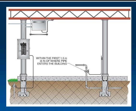
The building or structure grounding electrode system shall be used as the grounding electrode for a separately derived system (whichever is present and regardless of its nearness)
