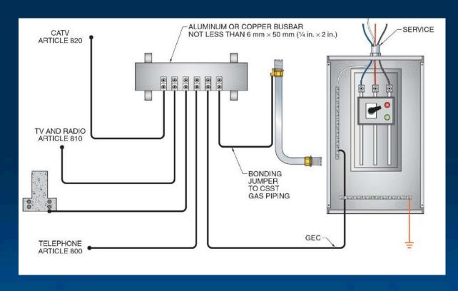
**250.94(B) Other Means.** Connections to an aluminum or copper busbar not less than 6 mm thick × 50 mm wide (1/4 in. thick × 2 in. wide) and of sufficient length to accommodate at least three terminations for communication systems in addition to other concerns.
